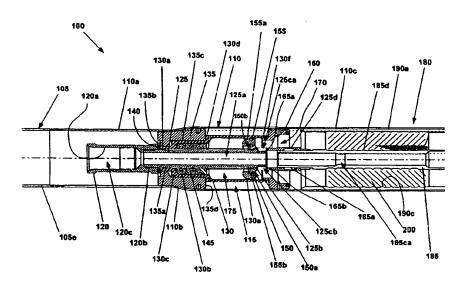
(57) Abstract: An apparatus (100) and method for forming or repairing a wellbore casing by radially expanding a tubular lincr (105).
